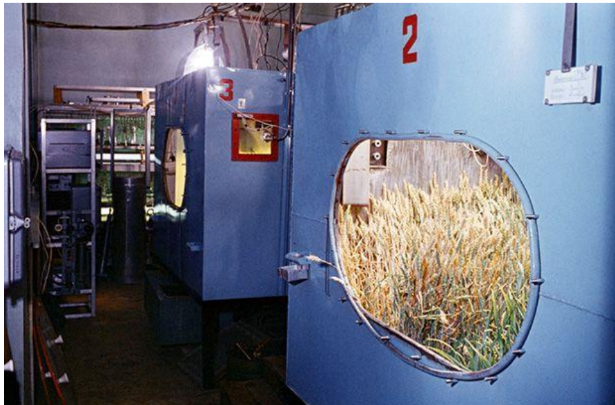
Figure 23 Bios-2 Algal Cultivator and Phytotron (Sohail, 2015)
